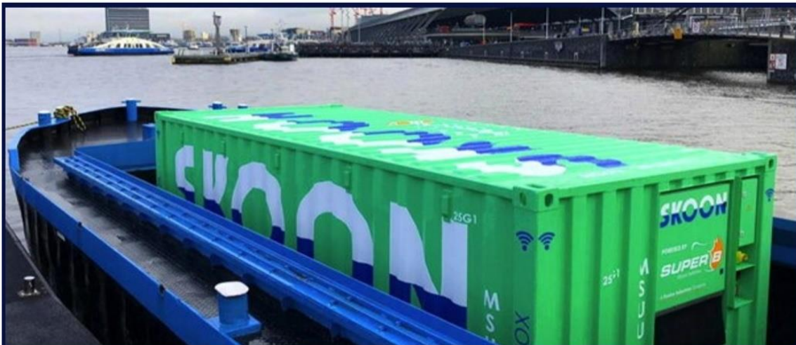
Shore batteries can be hired when there is only temporary need of shore power Commercially available batteries can provide up to 2 [MWh] of power in a 20ft container
