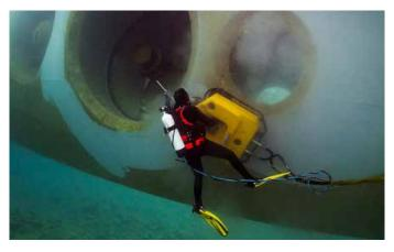
"Ecospeed with regular hull cleaning was a solution that worked for this cruise ship owner. The improved performance led to lowered fuel costs and CO2 emissions."
