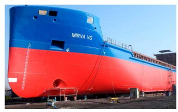
"The Ecospeed solution was the most effective coating system for reducing drag. With a hard coating we are also permitted to clean the hull underwater in the ports where we operate without damaging its waters and sediments."
