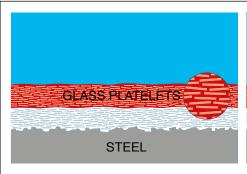
Two identical layers applied on the prepared surface make an impermeable barrier.
