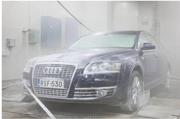
Figure 4. Testing of cold properties with diesel cars in a climate chamber.
